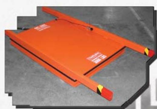
<The whisker switch ensures proper cart positioning
